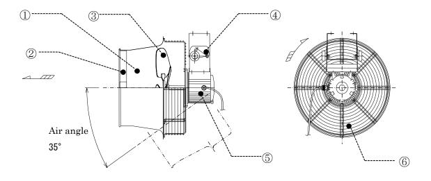
\* For 3 Phase motors, terminal box is attached instead of lead wire.
