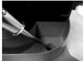
When inspecting or replacing the demister or filters, check for cutting chips in the drain pipe. If detected, remove the chips by hand or using a rod of no more than  $\phi 8$  mm in diameter. Clogging may prevent oil from draining properly.
