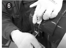
When securing the lid to the filter case, hold down the arm of the clamp to the lid with one hand as shown in the picture, then tilt the lever down to secure. (\*Make sure the arm properly sits back.)
