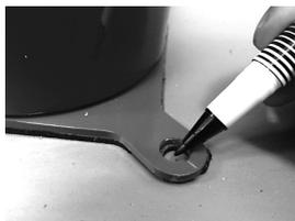
The centers of the installation holes marked in 4 and 5 can also be marked without doing any measuring, by drilling the holes marked in 1, 2 and 3, loosely anchoring the Mistresa and then tracing the holes. However, move the Mistresa out of the way to drill the  $\phi 10$  holes.
