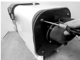
Insert the end demister (end filter) into the filter frame and lock the side cover in place with the truss screws. (With S model Mistresas, insert the end filter with the seam to the bottom.)
