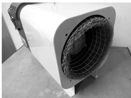
Remove the screws that lock down the side cover and detach the side cover so that the end demister (end filter) is visible.
