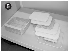
Install the replacements in the order of the secondary filter, space net, and primary filter. For the primary filter (2 pieces) and the secondary filter (2 pieces), put each one piece of them in place at a time with the stamp "Mistresa Genuine Part" facing the downstream (downstream of air flow direction). (Do not attempt to put all of them in at one time. Otherwise, you may not be able to install them in the right position.)
