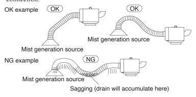
4 Positioning the intake port too close to the mist generation source could result in large amounts of mist, cutting chips, and dust to be sucked in, causing blow leakage and accelerated clogging of the filters and demister. Either provide an adequate distance (approx. 500mm) between the mist generation source and the intake port, or install an impact plate to prevent clogging from sucked-in mist, cutting chips, and dust.
