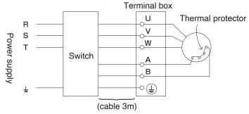
(5) Check the rated current shown on the nameplate of the Mistresa and set the thermal current to the rated current.
