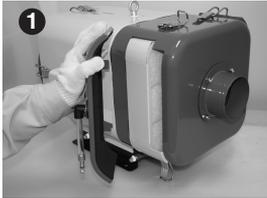
1 Unclamp the filter. Remove the cap.
