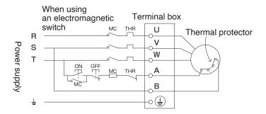
b) Connection example when using the optional switch with built-in 3SW thermal and a 3m cable)
